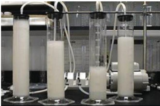
Figure 1 | A recirculation test is used to evaluate three defoamers in a semisynthetic fluid. The first cylinder on the left is a control run without defoamer while the best performance is seen in the third cylinder from the left. (Figure courtesy of The Münzing Group.)
